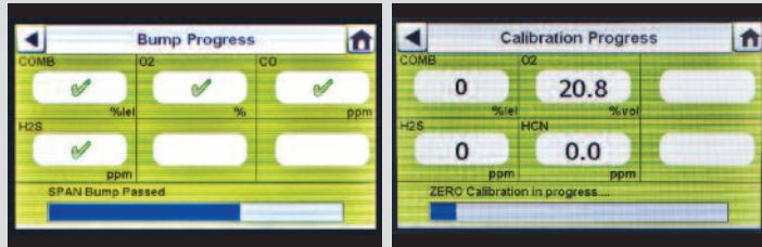
For **Bump** progress screen, hourglass symbol displays in each sensor box until that sensor's bump is complete. Green checkmark (✓) or red X (✗) displays for each sensor when bump test is complete.
