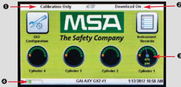
**Administrator** screen provides configuration options for the test stand, instrument & test gas cylinders:
